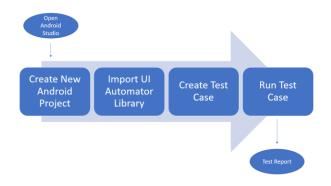
Fig. 1 Test Flow using UI Automator
